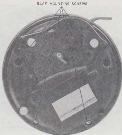
Fig. 2—881A105 (MD), 881A106 (MD), 881A107 (MD), or 881A108 (MD) Telephone Set, Bottom View
