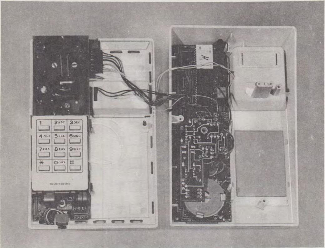
Fig. 5—5001T01A Telephone Set With Upper Housing Removed
