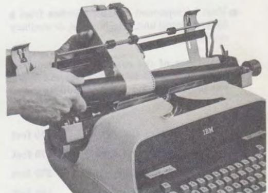
Fig. 9—Placing 1B Cartridge in Typewriter
