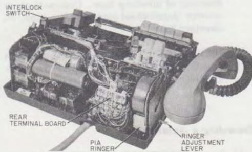
Fig. 7—2671B1M Telephone Set, Rear View
