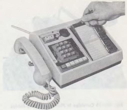
Fig. 8—Removal of 1B Cartridge
