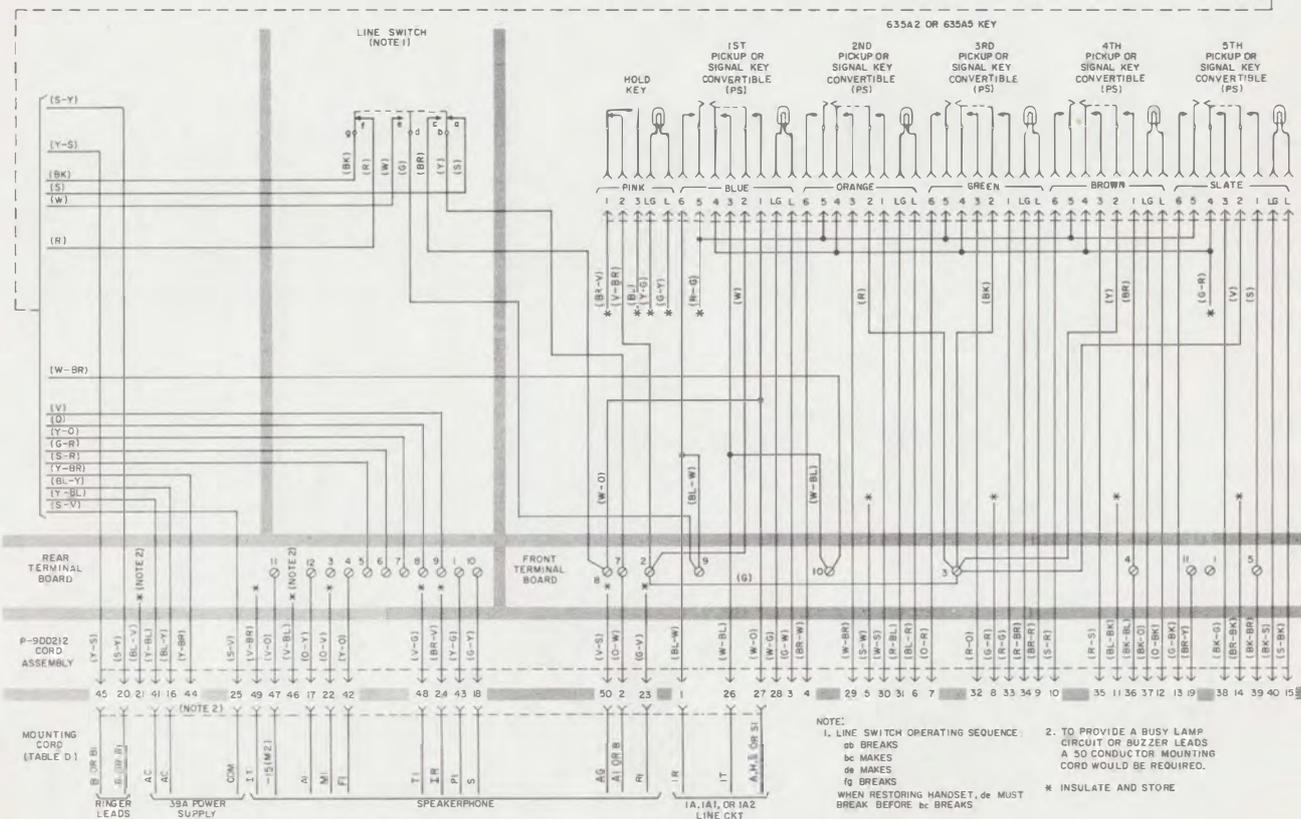
Fig. 13C—2671B1M Telephone Set, Wired for Single Line Service
