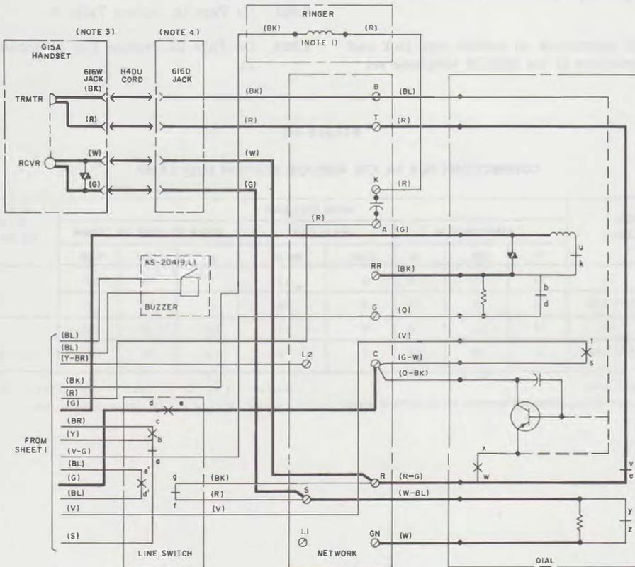
Fig. 29—2851CM Telephone Set, Connections (Sheet 2 of 2)
