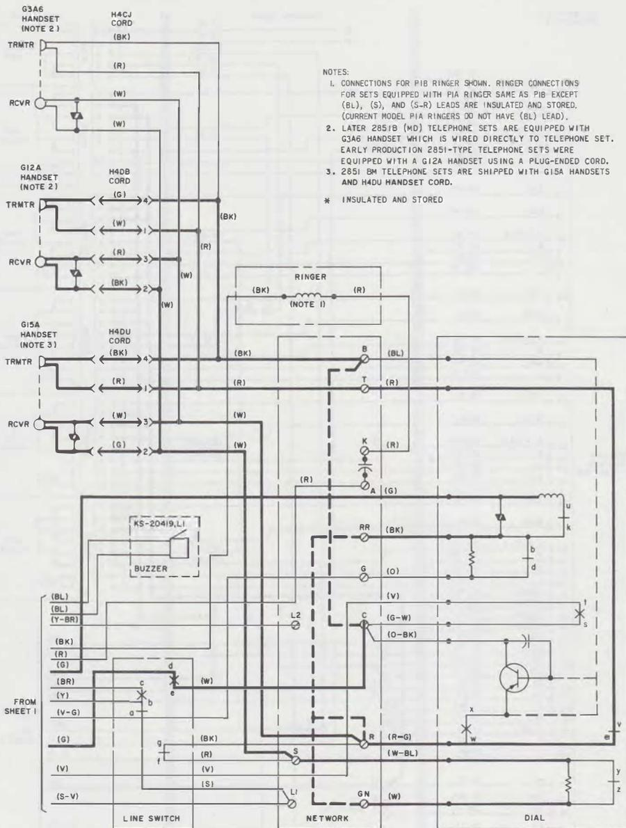
Fig. 27—2851BT, 2851B, and 2851BM Telephone Set, Connections (Sheet 2 of 2)
