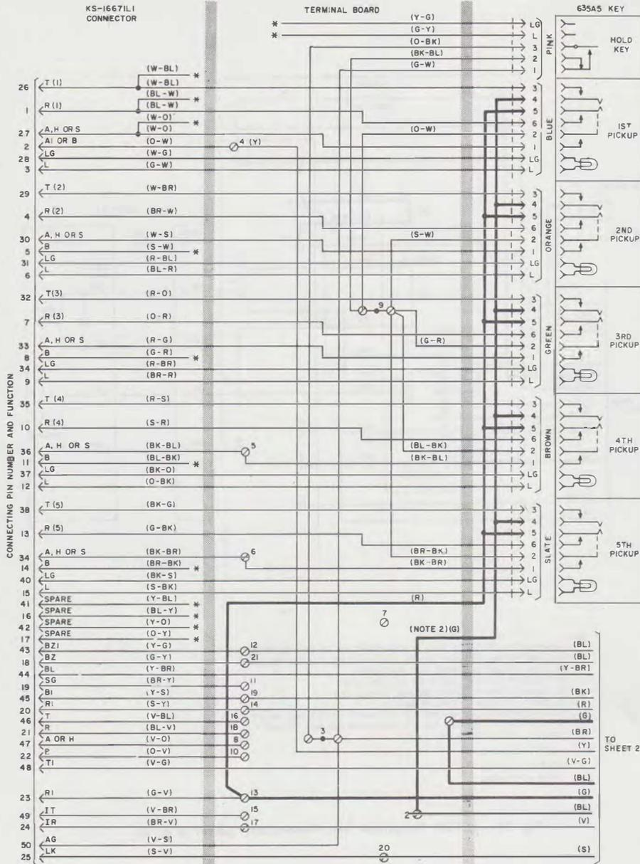
Fig. 29—2851CM Telephone Set, Connections (Sheet 1 of 2)
