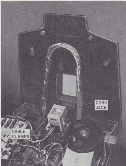
Fig. 7—Inside Wiring Cable, Exposed Wiring (Early Version)
