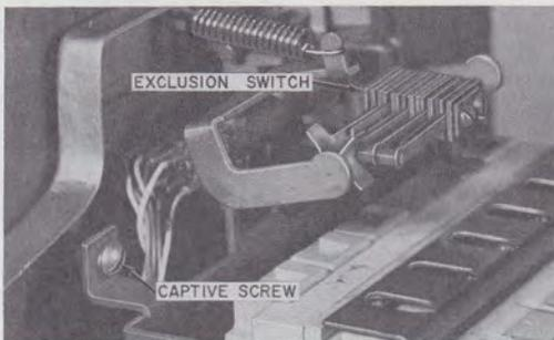
**Fig. 10—Exclusion Switch Installed and Hinged Chassis Mounting Screws (Early Version)**
