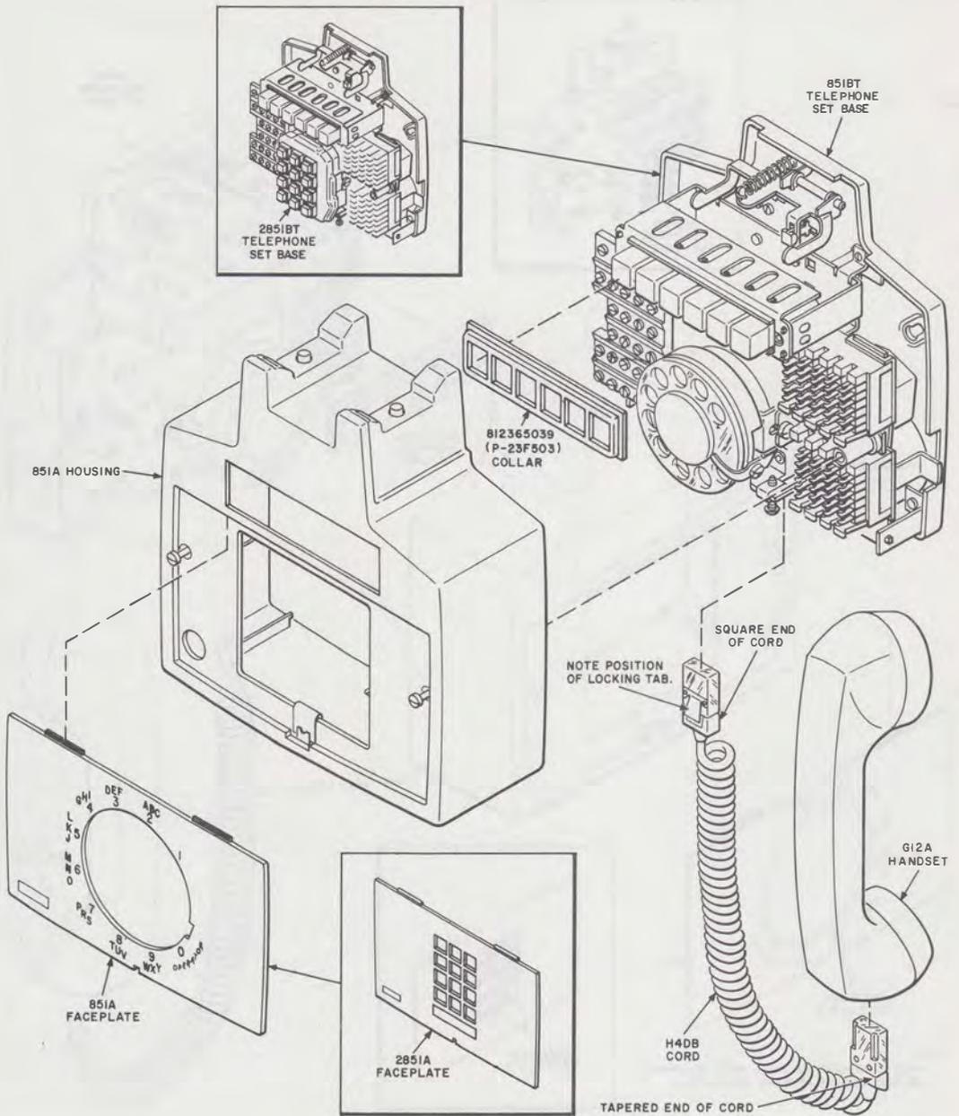
Fig. 19—Station Modular Arrangement, 851BT and 2851BT Telephone Set Showing Current 851A Housing and Base Plate
