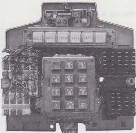
Fig. 4—Early Version 2851-Type Telephone Set Base (Housing Removed)
