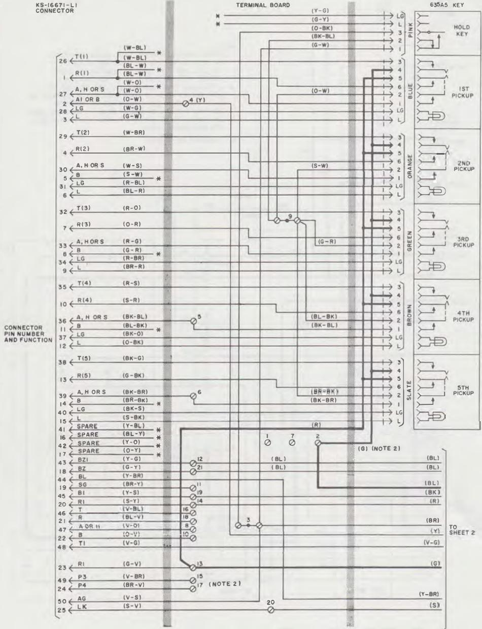
Fig. 28—851CM Telephone Set, Connections (Sheet 1 of 2)
