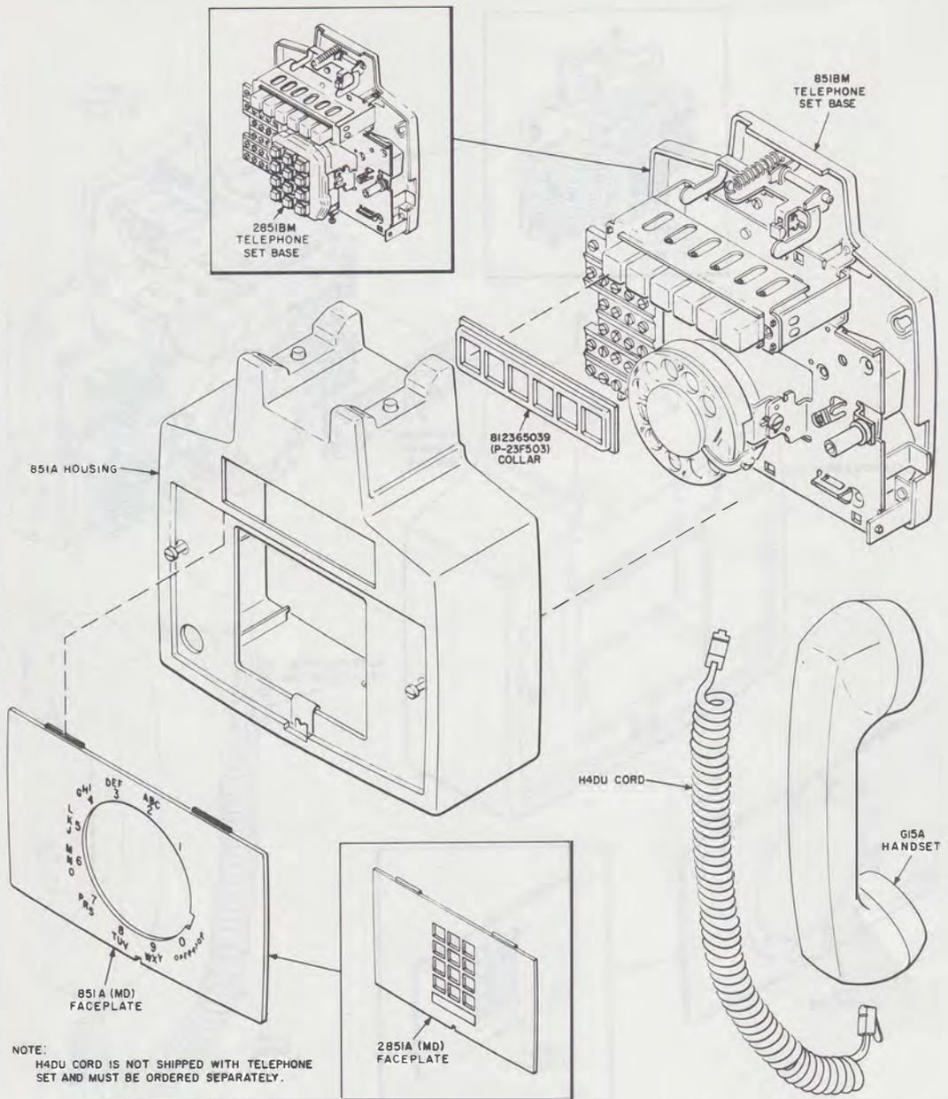
Fig. 20—Station Modular Arrangement 851BM and 2851BM Telephone Set
