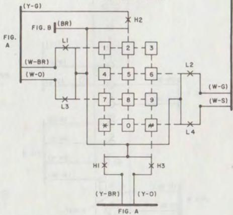
Fig. 8—2872A1M or 2872A2M Telephone Set, Connections (Sheet 3 of 5)
