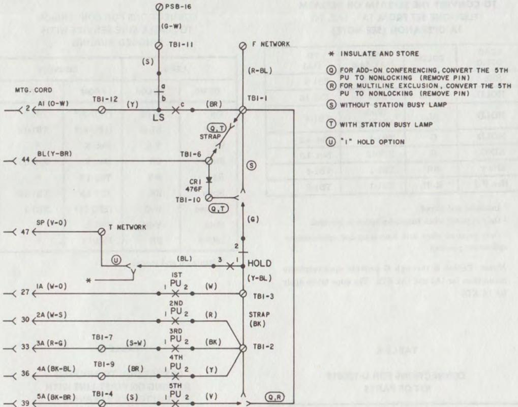
Fig. 9—"I" Hold, Exclusion, Station Busy Lamp, and Add-On Conferencing—TA1 and TA2 KTS (Showing 5th Key Modified)
