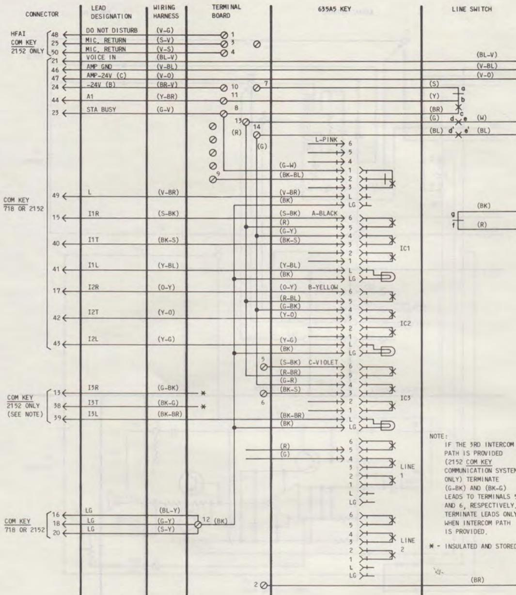
Fig. 7—2853AM Telephone Set, Connections (Sheet 1 of 2)
