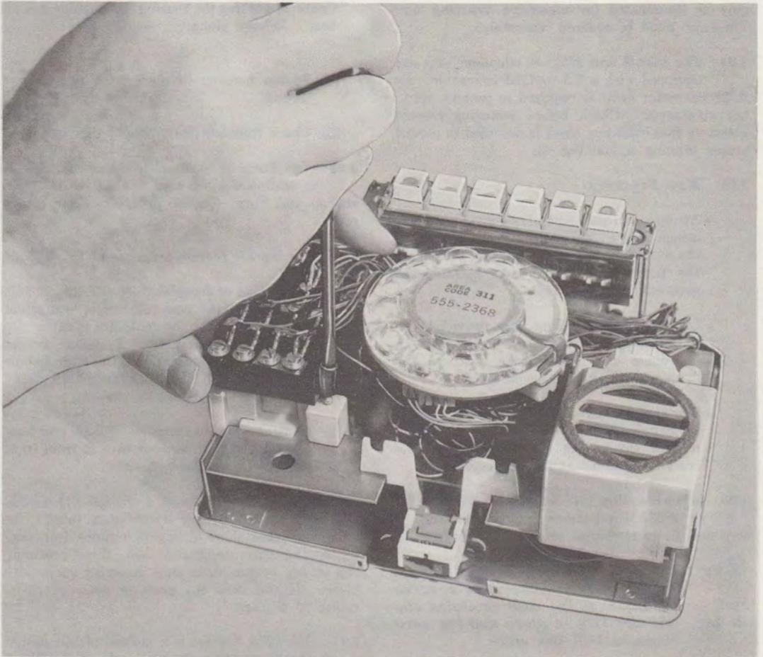
Fig. 4—Removing Terminal Board Mounting Screw
