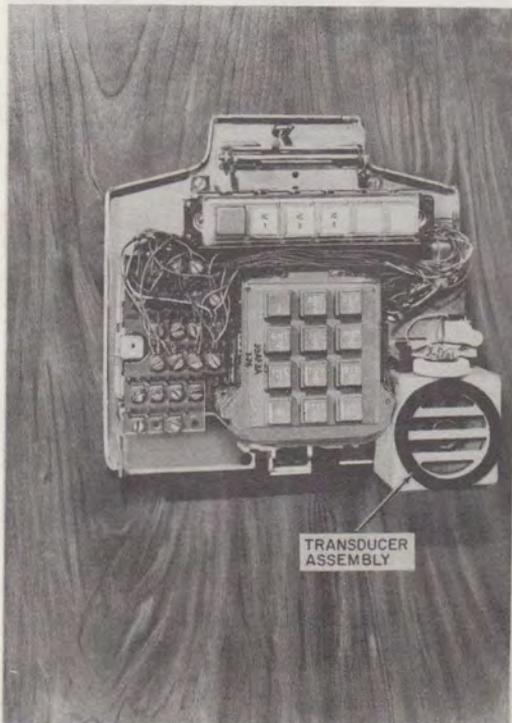
Fig. 2—2853AM Telephone Set (Housing Removed)
