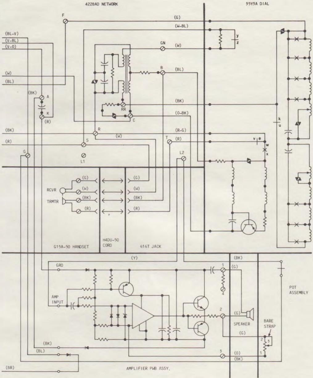
Fig. 7—2853AM Telephone Set, Connections (Sheet 2 of 2)
