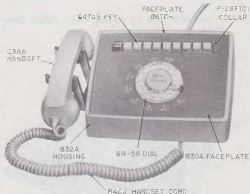
Fig. 1—830-Type Telephone Set, Assembled
