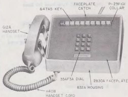
Fig. 2—2830-Type Telephone Set, Assembled
