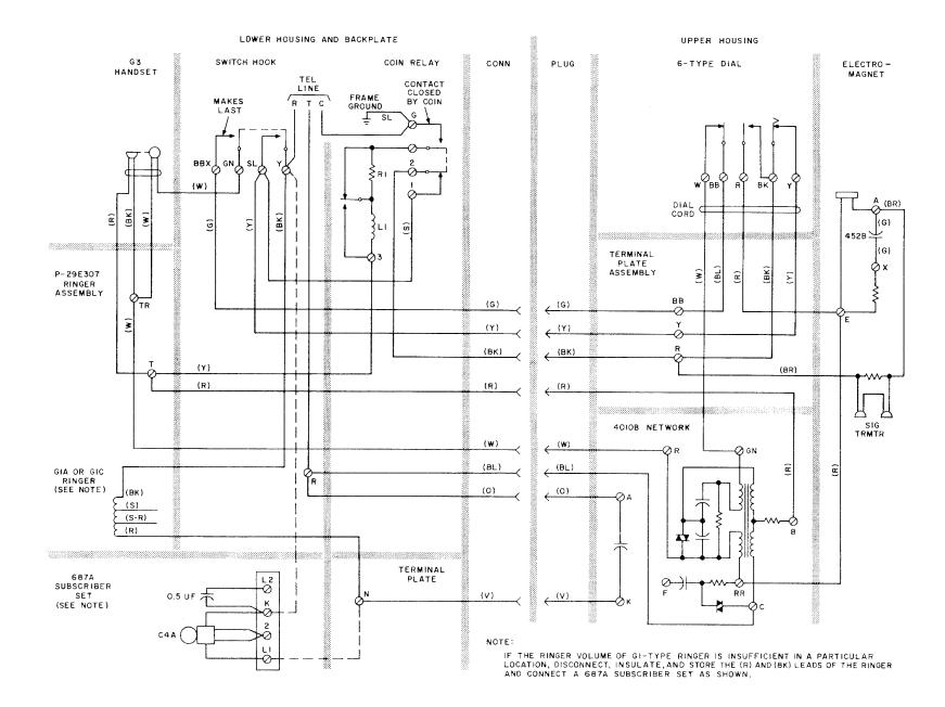
Fig. 1—236G Coin Telephone Set Connections
