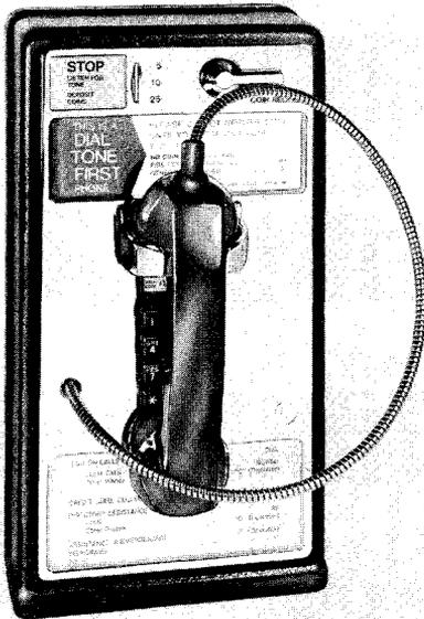
Fig. 37—Coin Cover Unit With Handset Inverted
