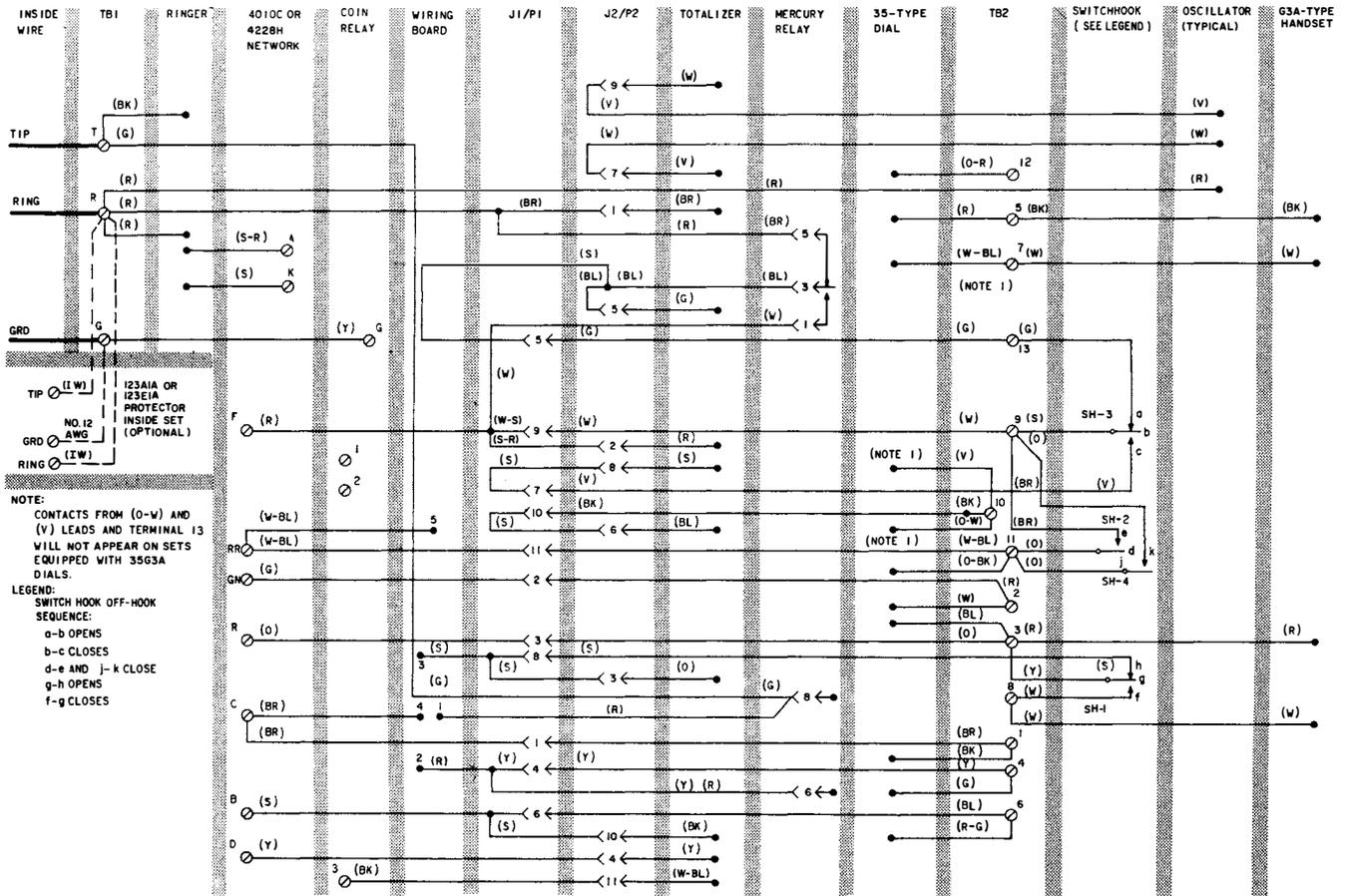
Fig. 65—1A2 or 2A2 Coin Telephone Set W/35T3A Dial—Connections
