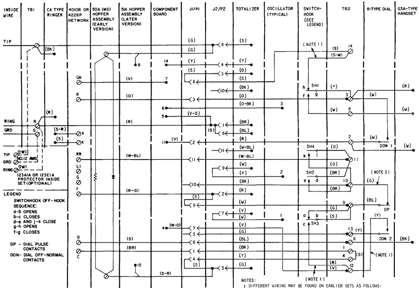
Fig. 73—1E1 Coin Telephone Set—Connections
