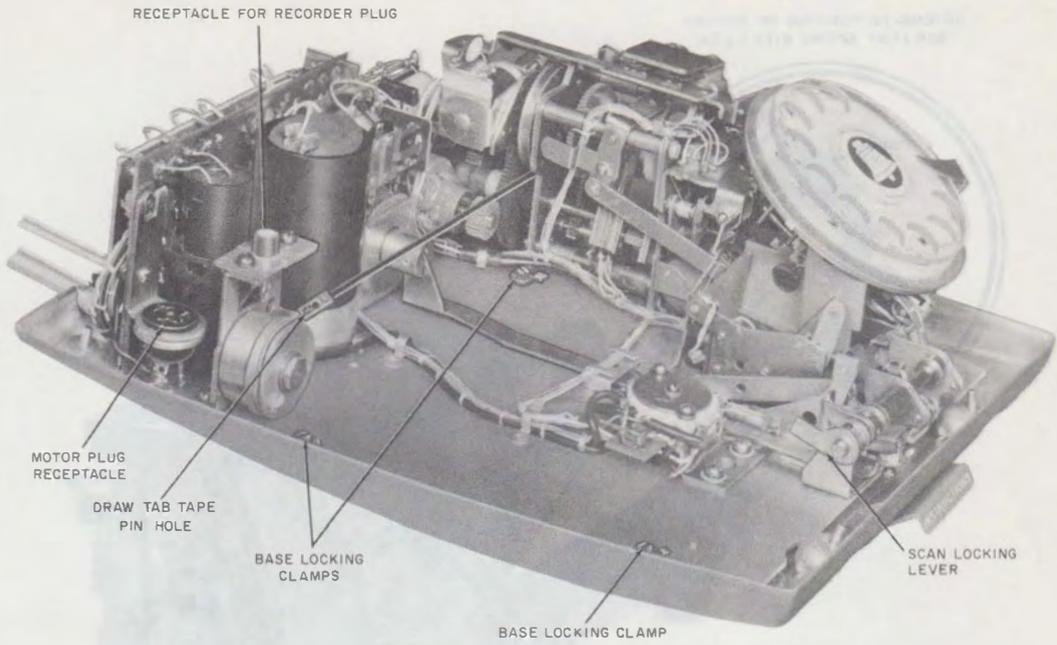
Fig. 10—KS-16844 List 10 *Rapidial*, With List 12 Tape Assembly Removed
