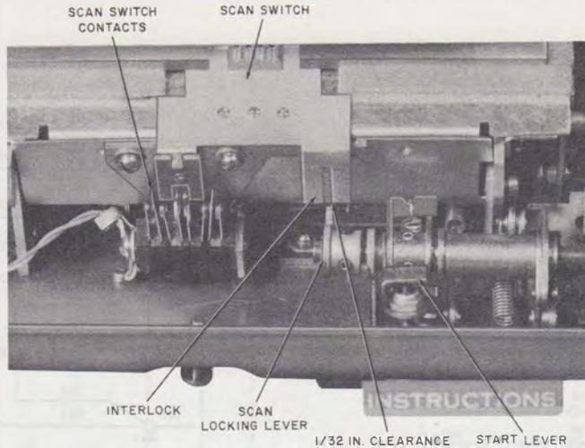
Fig. 12—KS-16844 List 10 *Rapidial* Start Lever Mechanism
