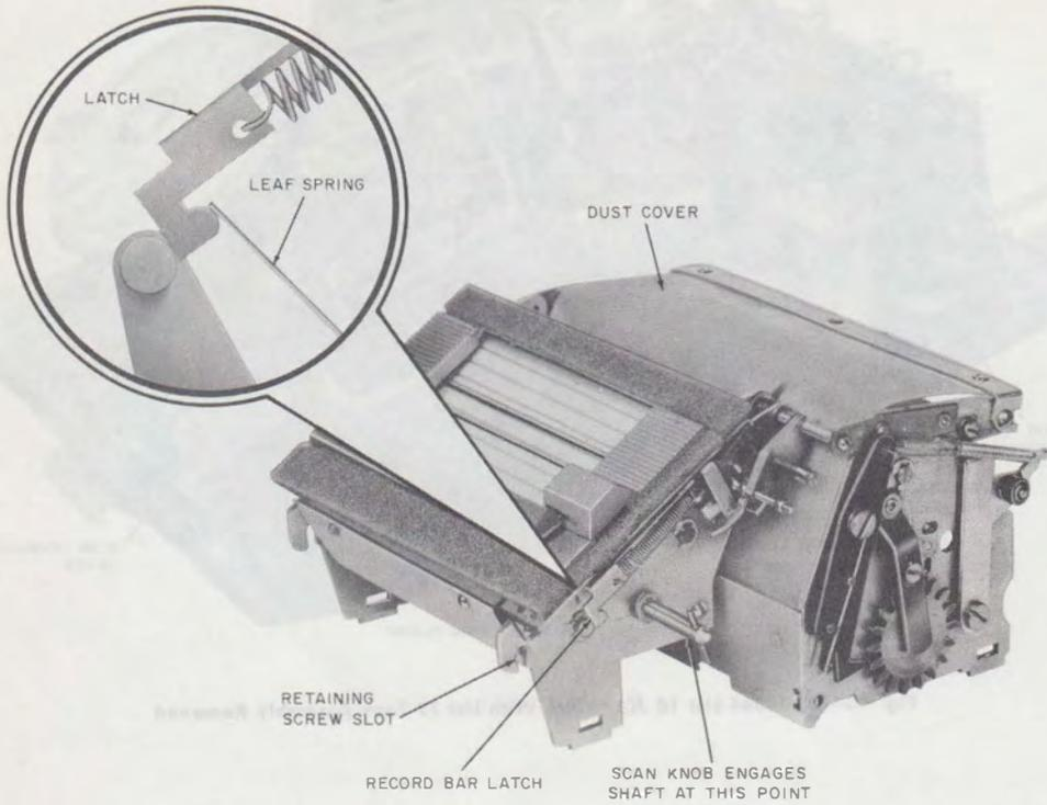
**Fig. 11—List 6 Tape Assembly (Front View)**
