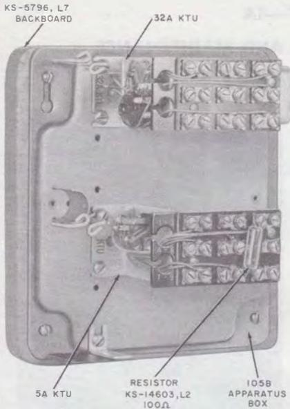
**Fig. 2—Battery Feed Filter and Holding Relay Equipment**
