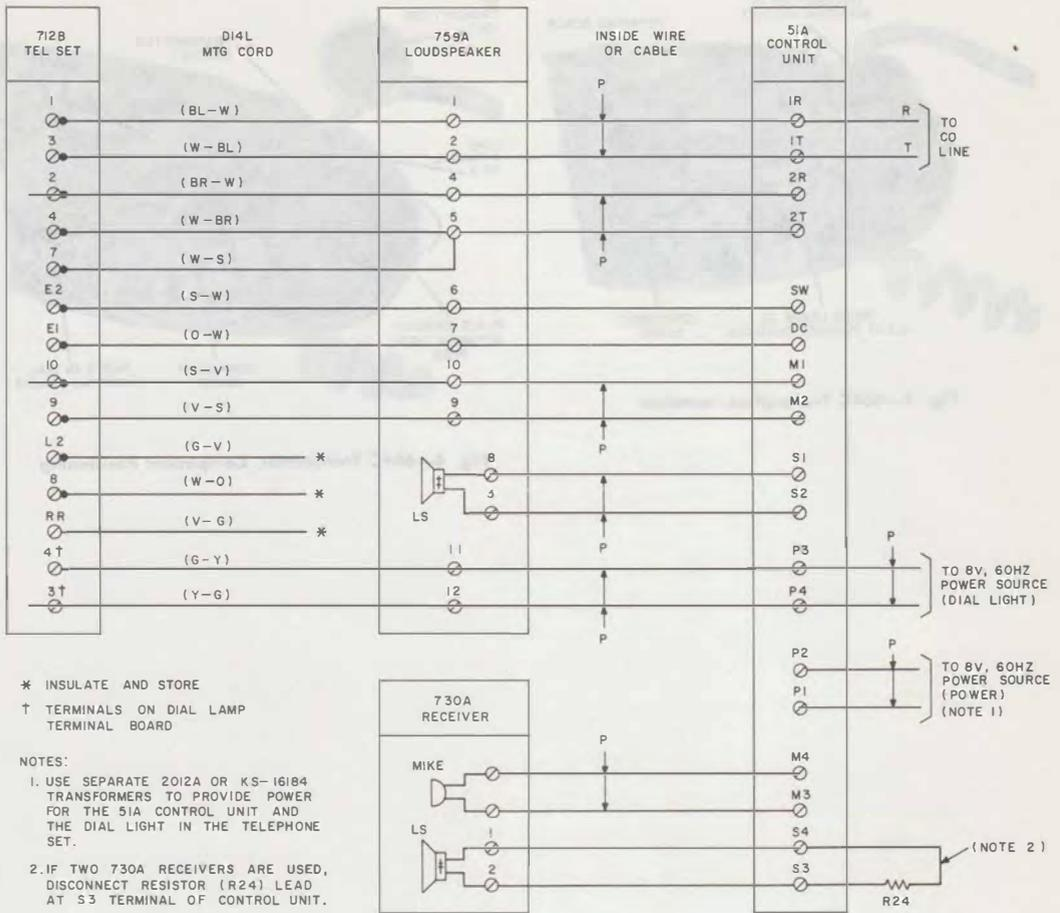
Fig. 2—712B Telephone Set, Connections to 1A Home Interphone
