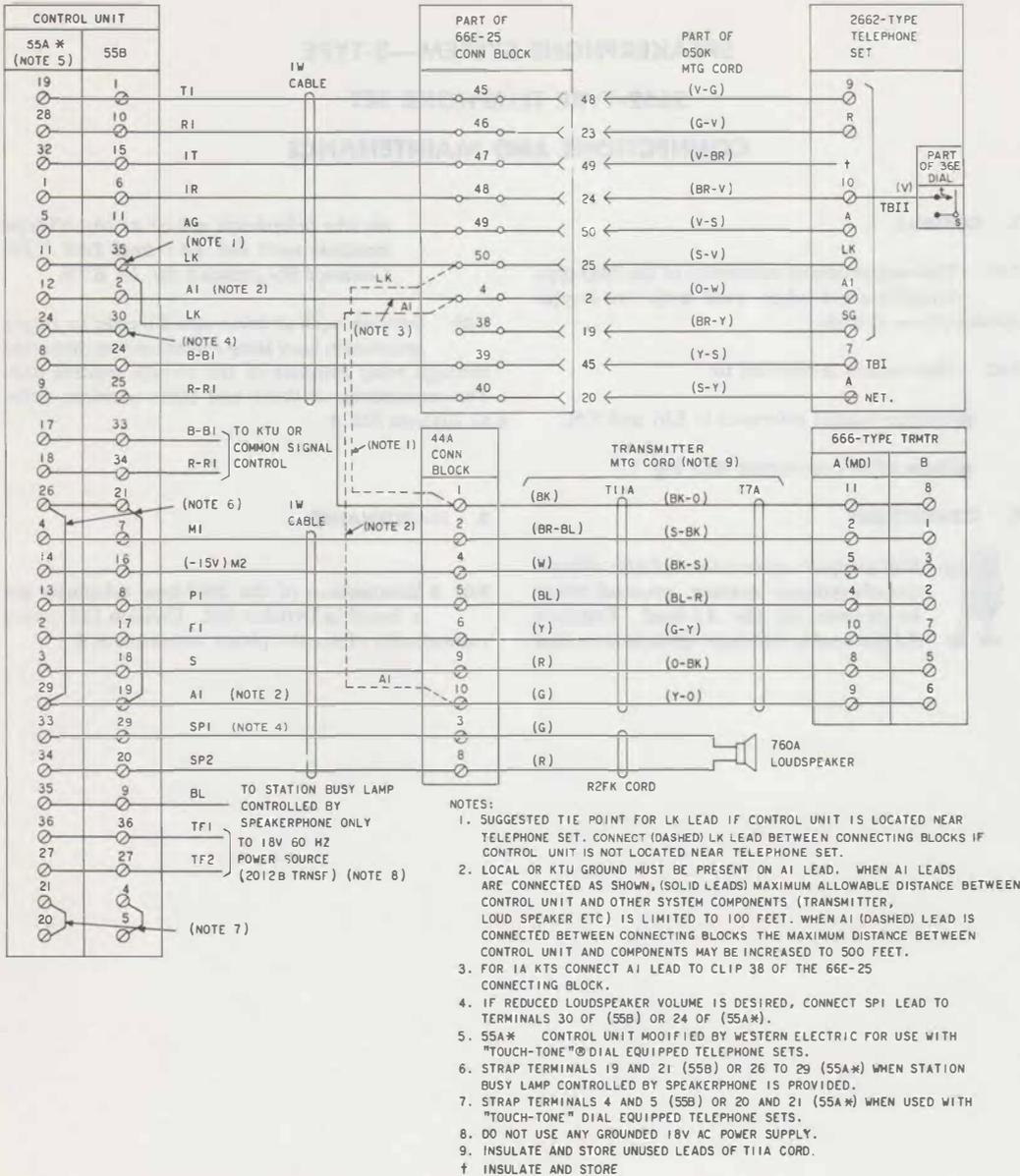
Fig. 1—2662-Type Telephone Set, Connections to 3-Type Speakerphone
