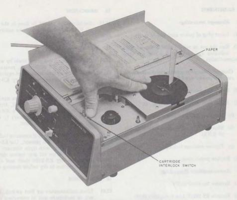
Fig. 7—Resetting "0" Registration on Message Indicator Dial
