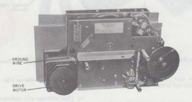
Fig. 6—KS-19245, List 3 Recorder (Motor Side)
