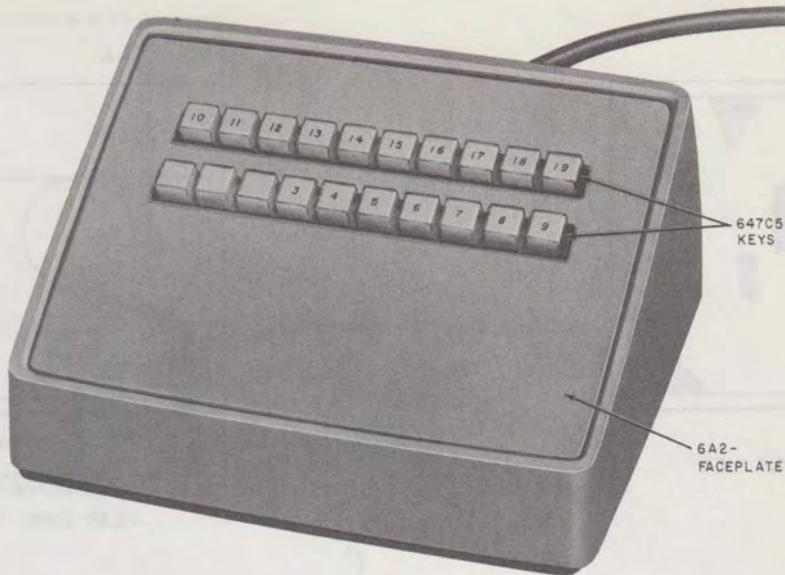
Fig. 8—6B1 Selector Console (MW)
