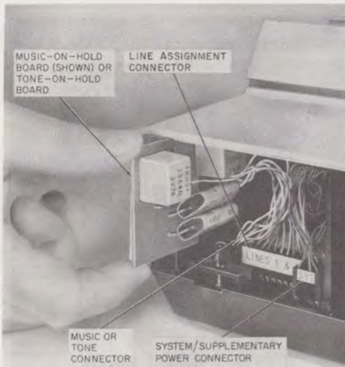
Fig. 21—Primary Set, Rear View With Heat Sink Removed
