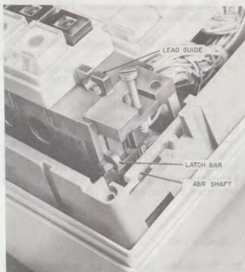
Fig. 58—Line Key Installation
