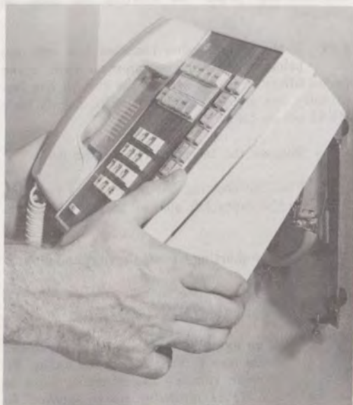
Fig. 18—Mounting Wall Set on Wall Plate
