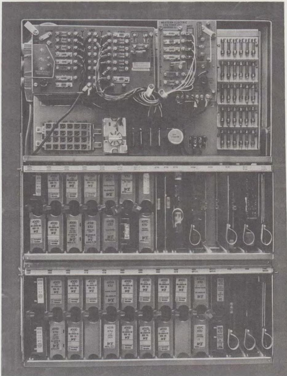
Fig. 2—121B Apparatus Box, Equipped With 2-Type Power Panel, 702- and 703-Type Feature Panels
