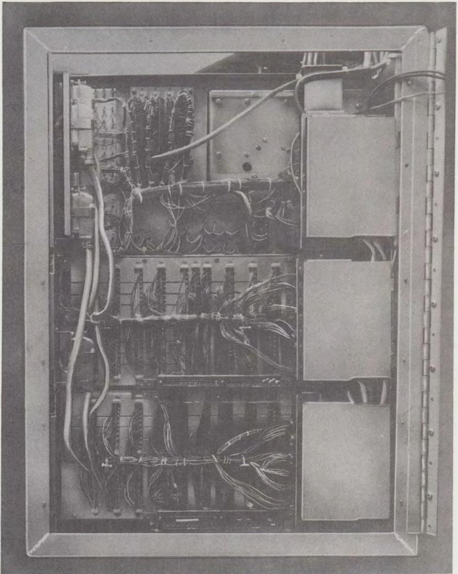
Fig. 3—121B Apparatus Box, Rear of Gate Assembly
