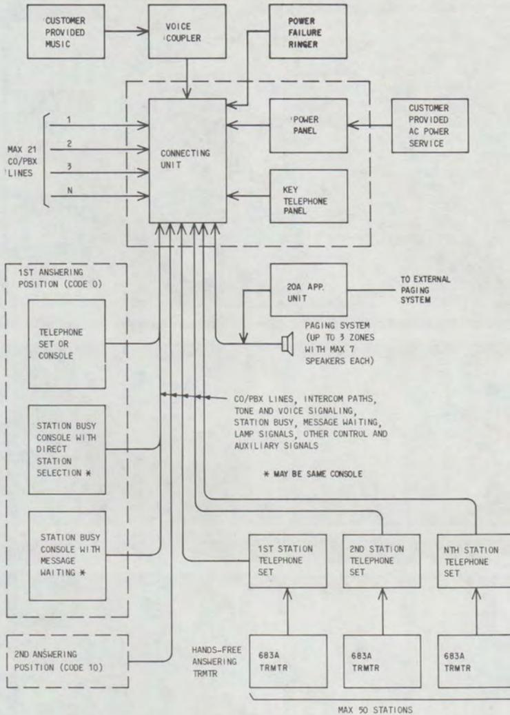
Fig. 1—Block Diagram of 21A Communication System
