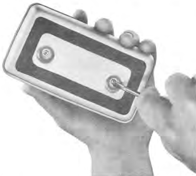
Fig. 20—Removing Housing and Panel Assembly From 72A Control Unit
