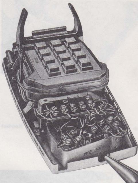
Fig. 19—Modifying 2554B-Type Telephone Set Base to Accommodate Handset Jack
