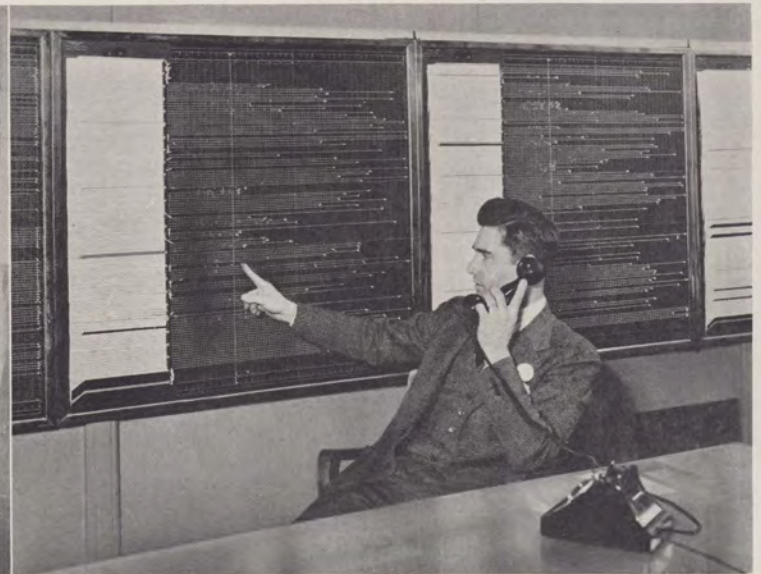
In a factory making parts for other war plants, this production control board shows the status of each order in process. Information on each job is made possible by telephone communication between foremen and the supervisor shown here. Different colored pegs indicate the date on which the job is scheduled to be finished and its present status.
