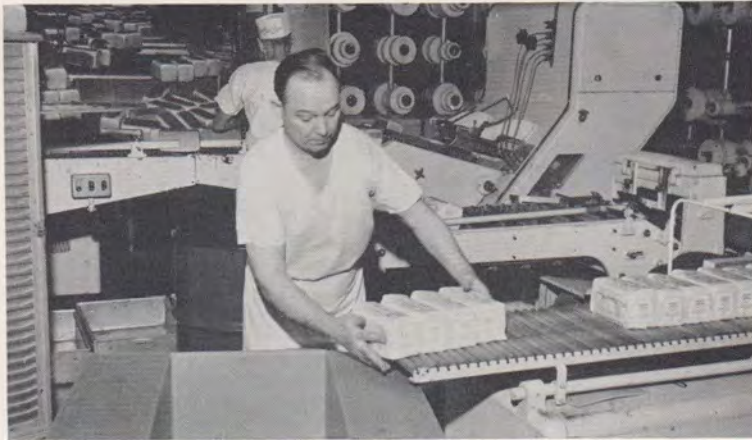
Loaves of bread make their hour-long cooling trip to the cutting and wrapping machine in Bakery. Batter for bread is mixed at 5:00 a.m., and bread is wrapped by 2:00 p.m.
