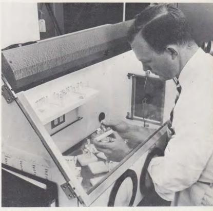
A Bell Telephone Laboratories engineer uses a "dry box" to assemble the new ultra-high-frequency transistor. He is shown placing a metal casing over the transistor to assure long life. Miniaturized electronic equipment is assembled in "dry boxes" to avoid contamination by dirt or moisture. The new transistor can withstand as much as 100 volts over a wide range of frequencies.
