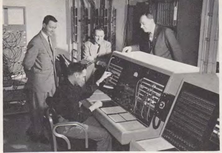
A data circuit patching panel (left) and a recording panel (right) have been engineered and installed by the N.E.T.&T. Co. for Lincoln Laboratory's SAGE Experimental Subsector. Standing: E. H. McGinnis, Technical Rep.; D. J. Hartrey, Comm. Eng.; and W. P. Norcross, S. & S. Mgr. H. J. Geisert, Lincoln Laboratory, is seated.
