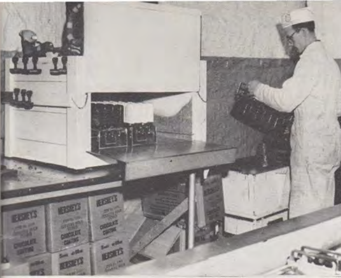
Two down and one to go. After the ice cream is "quick-frozen" on the stick it is taken out of the freezer and dipped in the deep brown chocolate liquid and then rushed back into the freezer to become a solid iceberg.
